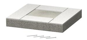
End piece for PYROLINE® Con S BSK fire protection duct, consisting of fibreglass lightweight concrete which is resistant to water and frost for closing the duct ends.
