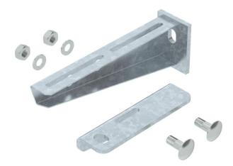
Bracket for mounting on suspended supports or as wall bracket for cable tray routing type above fire protection ceilings and for routing types with cable ladders and cable trays for the maintenance of electrical function according to DIN 4102 Part 12. The brackets are supplied ready-mounted.
