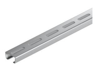
Central C profile rail for cable routing, in conjunction with clamp clips with a hammerhead foot. Can also be used as suspension construction for cable support systems.
