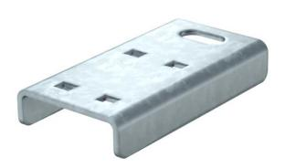
The connection component is the connection between the threaded rod lock and the suspension system for the routing types with cable trays for the maintenance of electrical function to DIN 4102 Part 12. Including bolts and nuts.
