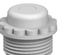
With perforation membranes, the opening D is pre-marked, but closed. Grip seal to screw into metric thread to IEC 423. With self-sealing cone at the end of the thread, therefore no connection thread
