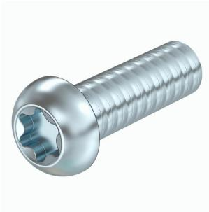
Flat head screw with TX 30, according to ISO 7380-1, suitable for fastening cable routes on brackets as well as for the mounting of barrier strips. The rounded head shape provides optimum cable protection. The Torx drive offers optimum force transmission in the screw movement.
