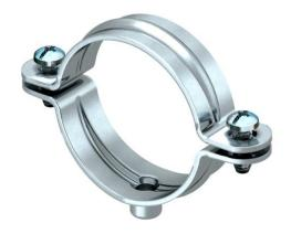
Mounting with screw-in spacer clips. Spacer clips and screw-in spacer clips are available in various materials: in V2A stainless steel, in electrogalvanised, hot-dip galvanised steel or in aluminium. Fastening can take place with bolt ties or angler anchors and Sprint screws.
