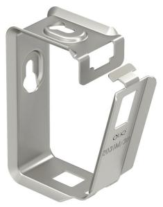
Metal grouped support for high mechanical stability, even in case of fire. Suitable for safe mounting above fire protection ceilings. Also approved as a cable-specific variant for the maintenance of electrical function to DIN 4102 Part 12. For wall and ceiling mounting. Lock can be opened without tools. Detailed information on the approved routing variants can be found in the appropriate testing documenta-
