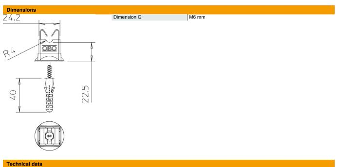
Holder fastening typeWith anchorConductor fastening typeWith clamp clipHigh voltage-resistant, insulated<br/>versionnoCable dimensions8 mm roundMounting height20 mm
